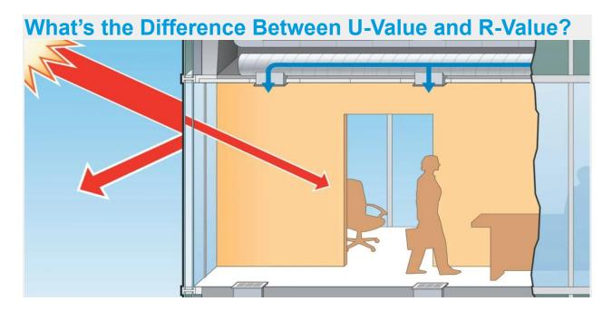
One of the most important glass performance measures is U-value—also known as U-factor—which measures the insulating characteristics of the glass, or how much heat flow or heat loss occurs through the glass due to the difference between indoor and outdoor temperatures.
